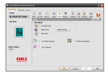
Fiery Expert Color settings (shown below) allow all aspects of the image/content to be fine tuned. Custom profiles, rendering intents and spot color matching can be applied here. For additional detail, please refer to the Fiery Color Technical Reference, the Fiery Printing for Windows (Mac) Reference, and the Fiery Print Options Guide on the CD.
