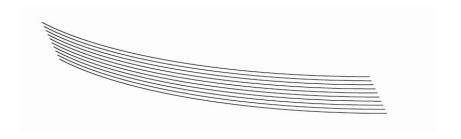
The 2" stack of media should be 'pre-shingled' (fanned and angled back on the leading edge). If media is loaded in this fashion from the start it will simplify adjustment and set-up of the feeder.
