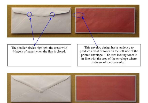
The images above illustrate that the pressure points of a particular envelope design may interfere with the printer's ability to maintain uniform contact between the printer's image drums and the surface of the envelope.
