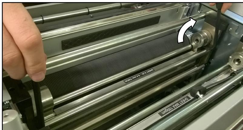
**9** Slide the blade assembly out of the creasing unit and lay it on a flat surface
