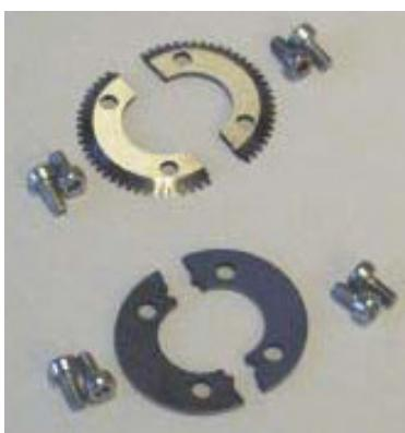
The perforator blades are split into two matching halves and are fitted to the drive wheels as shown in the photograph using the four screws supplied.
