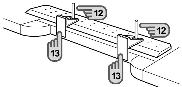
**13** Slightly loosen the knife handles and remove the knife holders.
