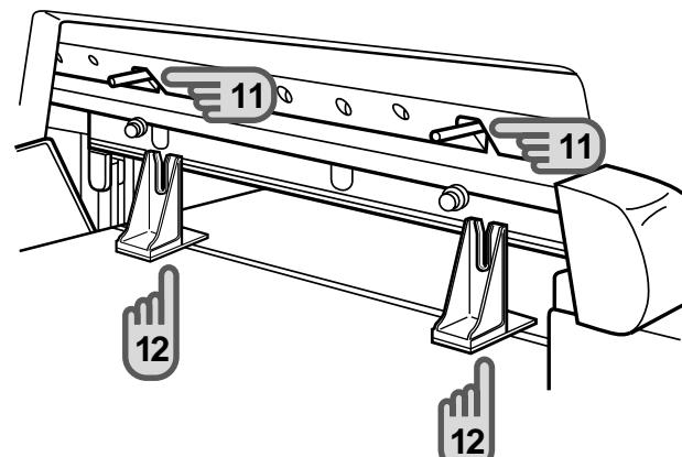
**14** Tighten the knife handles to fix them to the knife holders.
