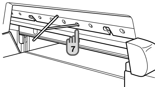
**7** Remove the knife installation bolts.
