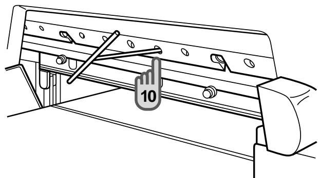
**11** Install the knife handles into the notches cut in the middle plate, while not tightening them.
