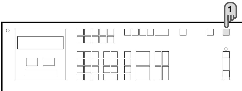
1 Turn the working lamp switch "OFF".
