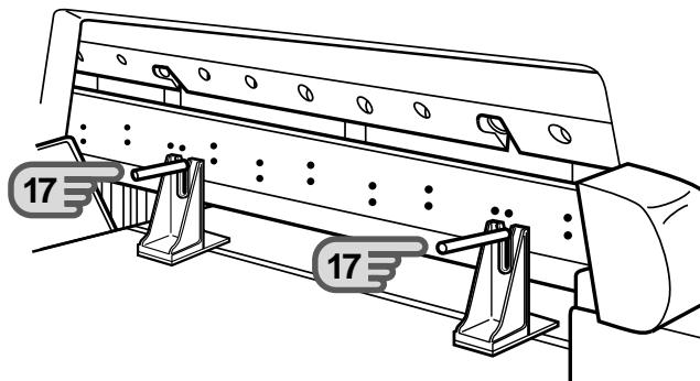
**18** While holding the knife handles, fall the knife on the leveling block.
