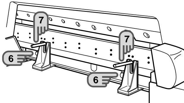
**7** While holding the knife handles, release the clamp pedal slowly to raise the clamp.
