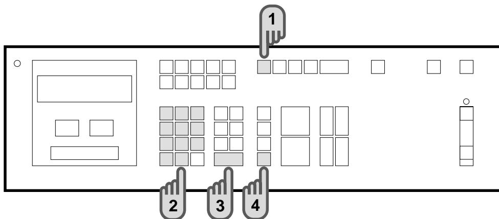
To let out air in the paper ream, send out the backgauge and lower the clamp only.
