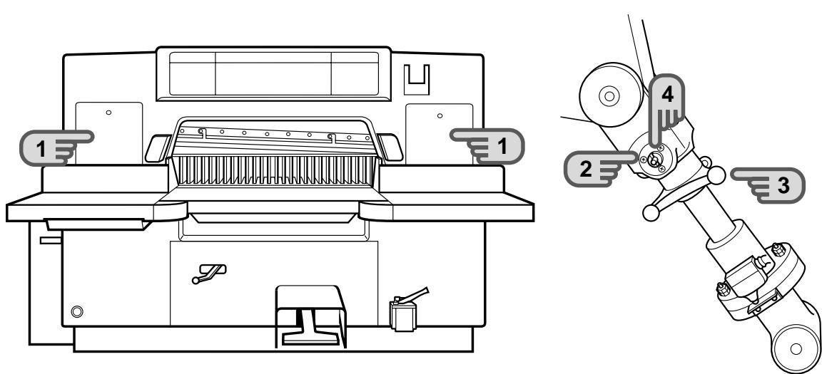
**1** Remove the lid of the knife height adjusting window.
