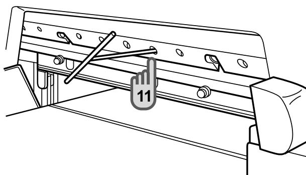
Do not install the bolt next to the leftmost one at this time.
