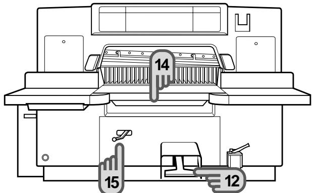
**15** Move the knife change lever into the CUTTING position.
