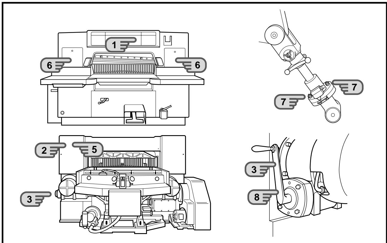
If a hard matter or foreign matter is cut or a dull knife is used to cut, the safety bolt will be broken to stop the knife in an emergency.
