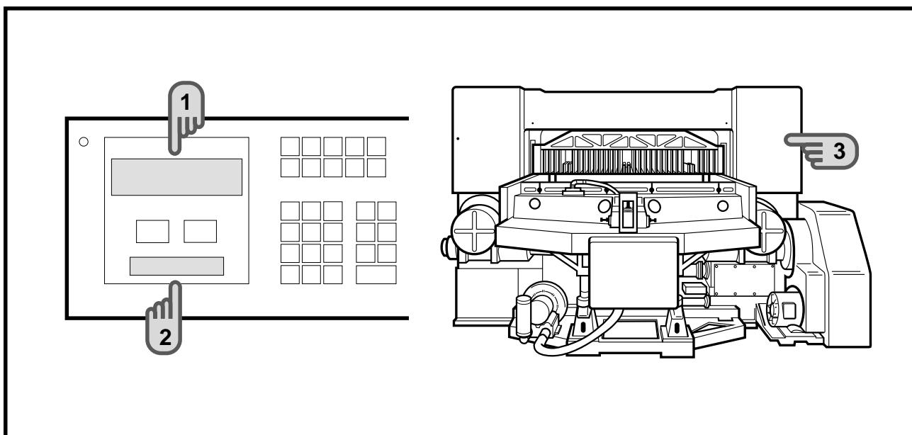
**1** When the thermal relay trips or the safety bolt is broken, error display appears.
