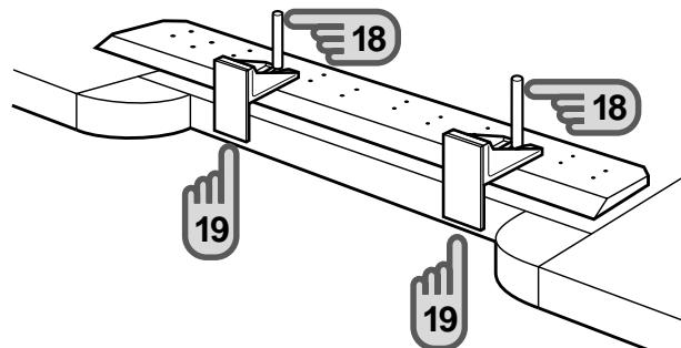
**19** Slightly loosen the knife handles and remove the knife holders.
